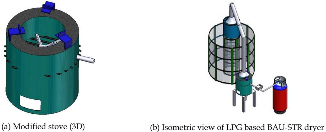
Figure 3. Development of LPG system as heating source for BAU-STR dryer
