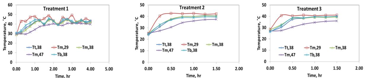
Figure 4. Drying air temperature variation of several treatments
