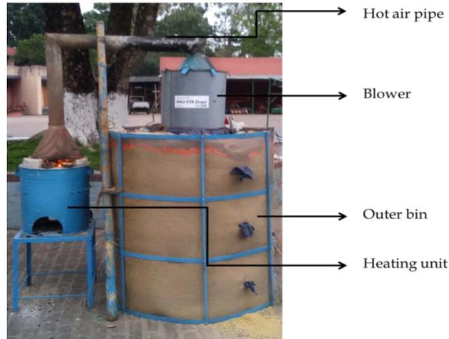
Figure 1. BAU-STR dryer
