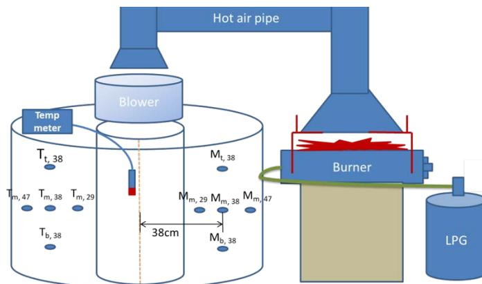
Figure 2. Experimental layout of BAU-STR dryer's temperature sensor placement and moisture measuring points (T-temperature sensors, M-moisture measuring point, t-top, m-middle, b-bottom, number in subscript indicate distance from the center line in cm).
